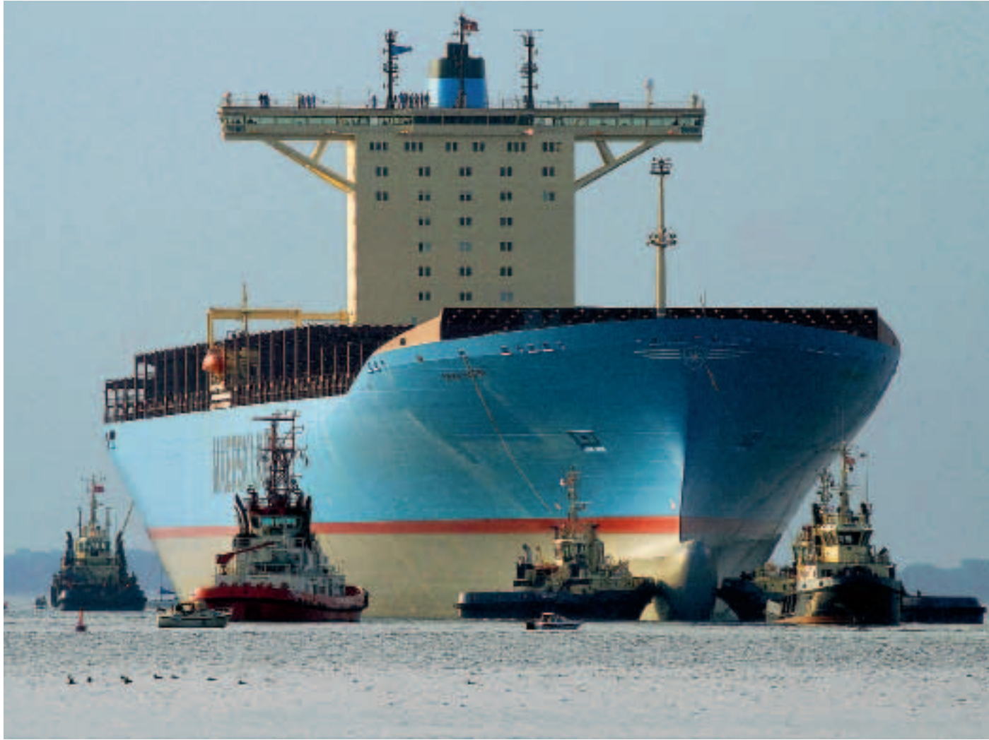
Emma Maersk is the world's largest container vessel, measuring 397 metres long, 56 metres wide and able to carry 11.000 TEU. Photo Maersk Lines 2006.
